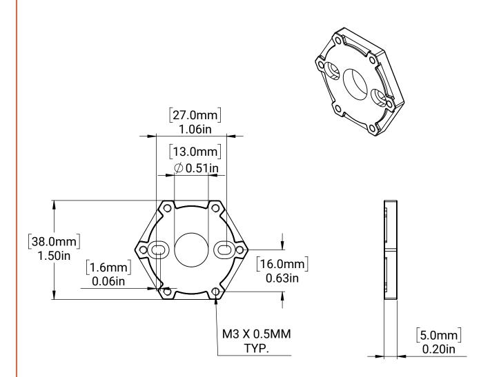
MM SHEET TOLERANCES: X ± 0.50 MM X.X ± 0.10 MM X.XX ± 0.05 MM ANGLES ± 2° INCH SHEET TOLERANCES: X ± 0.1 IN X.X ± 0.02 IN X.XX ± 0.004 IN X.XXX ± 0.002 IN ANGLES ± 2° MATERIAL:
